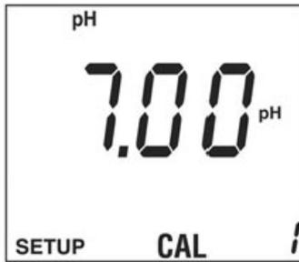
4. Push **ENTER** to set the first calibration buffer. The display will show the pH buffer for the next calibration point.
