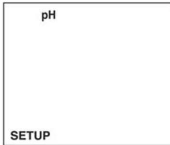
3. Push **ENTER**. The display will show the pH resolution. Use the arrow keys to set the pH resolution between 0.01 and 0.1.
