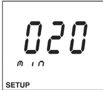
4. Use the numeric keypad or the arrow keys to set the shutoff time in minutes. Set to **000** for continuously on.
