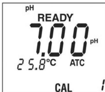
4. If the buffer is correct, push **ENTER**. The pH buffer value will flash until calibration is complete.
