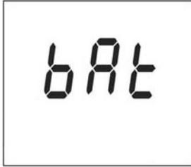
**Note:** Replace the batteries when the battery icon indicates about 25 hours battery life remaining.
