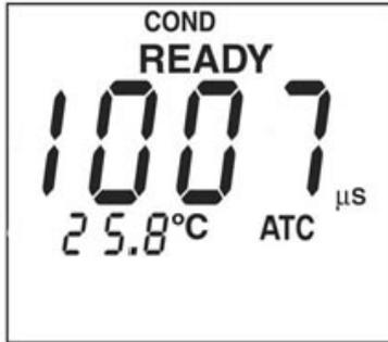
3. Push the arrow keys to scroll to the value of the conductivity or TDS standard and push **ENTER**. The main display and the wait icon will flash.
