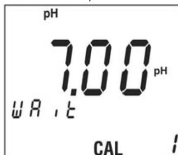
**Note:** Calibration can be stopped while the pH value is flashing. Push the **PH** or **SETUP** key to return to the measurement mode.
